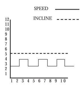
The **Cardio Program** is designed to vary the treadmill Speed, while maintaining a constant Elevation.
